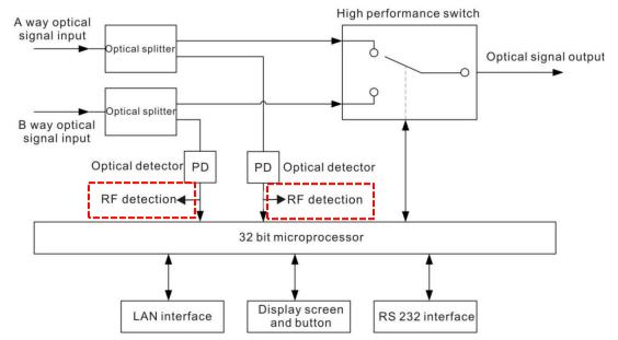
Note: The red dotted frame in the figure is only for enhanced optical switch.
